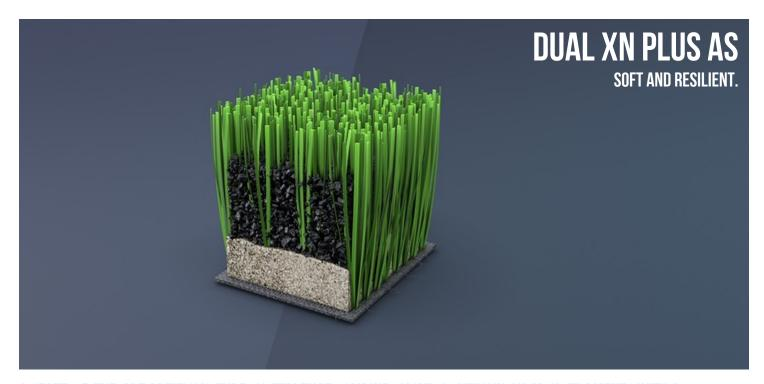
A STATE-OF-THE-ART ARTIFICIAL TURF SYSTEM THAT COMBINES MONDO'S NEW XNOVA MONOFILAMENTS WITH A PARALLELOGRAM-SHAPED STRUCTURE WITH CONCAVE SIDES THAT FORM 4 GROOVES AND 4 ASYMMETRICAL RIBS, 5NX MONOFILAMENTS WITH A SEMI-CONCAVE STRUCTURE WITH 3 ASYMMETRICAL RIBS, AND PERFORMANCE INFILL MADE OF SBR GRANULES.
